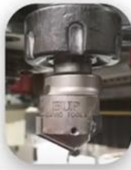
45° downcut end milling cutter
