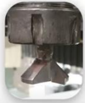
45° upcut end milling cutter
