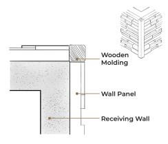
**Option 2:** Use a square piece of molding, running vertically, to join wall panels and create an outside corner with a special emphasis on the corner itself. We recommend that you use a complementary wood type and color for this solution.
