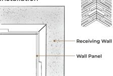
A seamless, inside corner can be achieved by joining panels using a miter joint.
