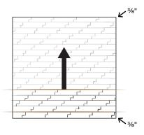
Continue to work bottom to top, left to right, as you add rows. After the installation of the first five rows, check that straight lines have been maintained, correcting if necessary.
