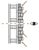
Where panels are to be installed onto a wooden receiving wall, a nail gun may be used as an alternative (or in addition) to an MS
