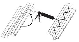
elastic MS polymer adhesive. As a guide, you will need one standard 10 fl. oz. tube of adhesive per 20 sq. ft. of paneling.
